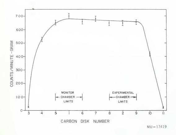
Fig. 9. Neutron beam structure determination using the  $C^{12}(n, 2n)C^{11}$  reaction.
